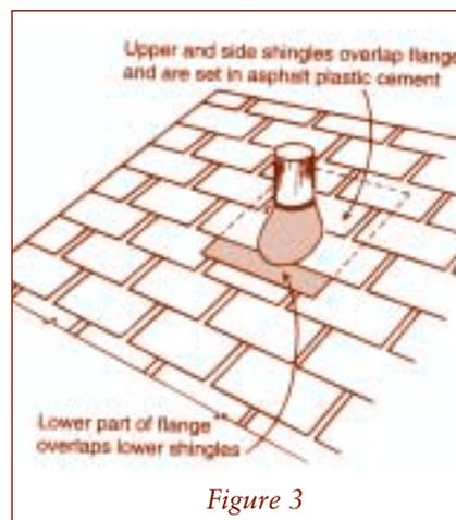
ceiling or caulk around the base of the boot at the shingles. Sealant in this area will often trap water and cause a back up of water cement under the shingles, and it is a sign of amateur workmanship. Sometimes an exposed flange is caulked to the shingles, but this should not be necessary if it is installed correctly. Its rubber seal can split and leak
